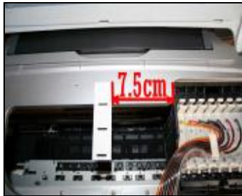
Stick the Support arm at 7.5cm distance from the side of the printer, Rip the
