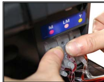
Press the cartridges make sure They contact well with printer
