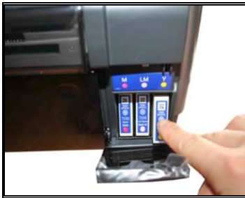
Press the cartridge, then Cartridge will come out
