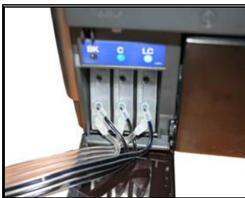
Install the other sides cartridges
