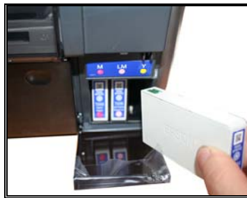
Remove the original cartridge
