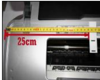
Stick the Support arm at 25cm distance from the side of the printer
