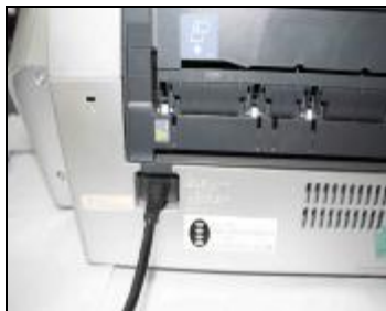
Insert the electrical source line suitably
