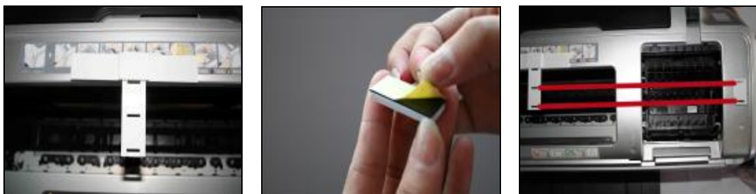
Stick the Support arm at 25cm distance from the side of the printer
