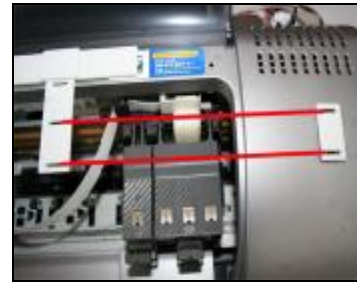
Rip the label on the balance arm
