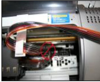
The tube is twist ,it is not ok.
