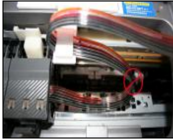
The tube is excessive long, it is not ok.
