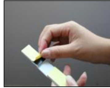
Rip the label on the balance arm
