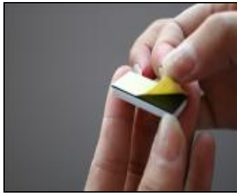
Stick the Support arm at 11.5cm distance from the inner side of the printer
