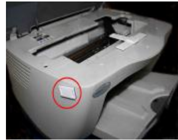
Attached the clamp at the top right of your printer
